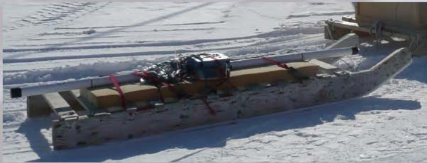
Figure 12: A photograph of the autonomous sea-ice thickness sensor deployed on the SmartQAMUTIK. The sensor is an adapted ground conductivity meter (Geonics EM31) that employs electromagnetic inductive methods to measure ice thickness.
